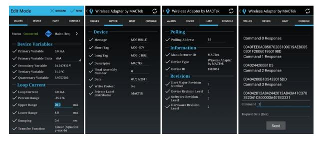
teknikol COMMANDER's most powerful feature is its engineering console. This allows the user to read or write any command, including device-specific commands and associated data. The engineering console enables full configuration of any HART® field device. The teknikol development team has put extensive development and testing into COMMANDER, including an open beta test before this public release. The team has also put together a limited free version, which is available on the Google Play store.
